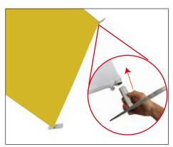
5. Attach the feet and stand the display up. Note: Feet should align to the outer edge of the frame.
